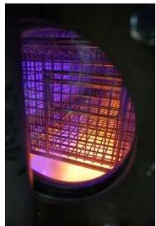
By adding low-pressure plasma cleaning to a wet chemical cleaning system, film-type contamination can be minimized for unsurpassed cleanliness.
